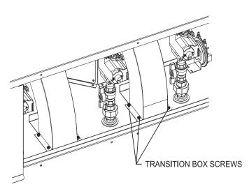
Figure 53 – Loosening Fan Transition Box Screws
